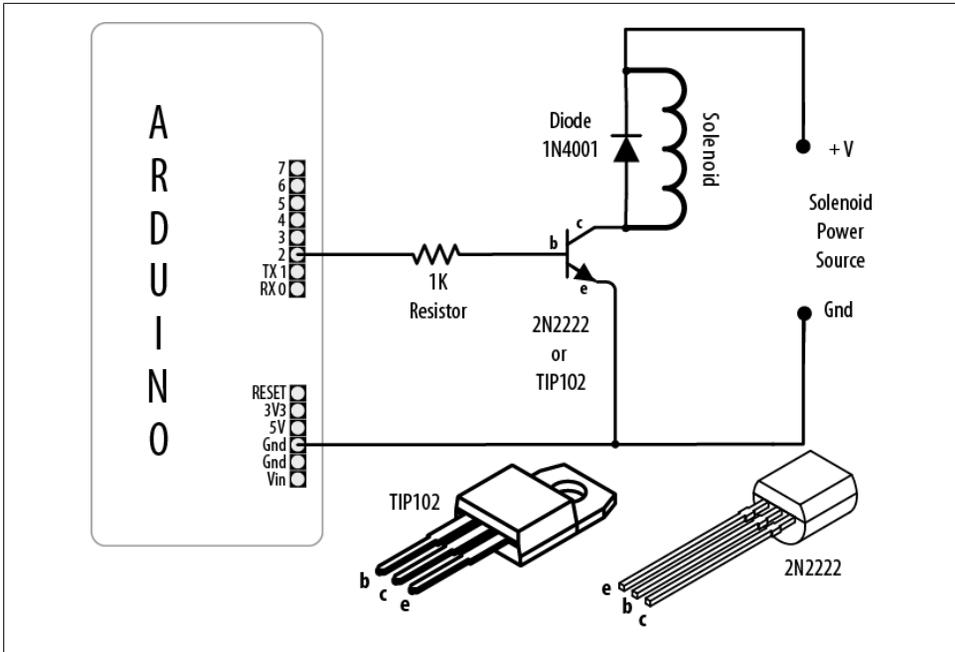
Figure 8-7. Driving a solenoid with a transistor
