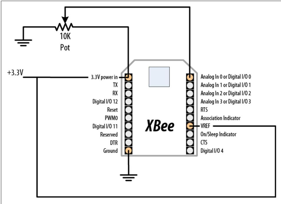
Figure 14-8. Series 1 XBee connected to an analog sensor
