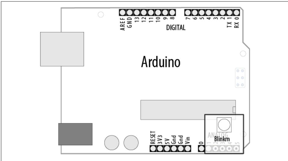
Figure 13-3. BlinkM module plugged into analog pins
