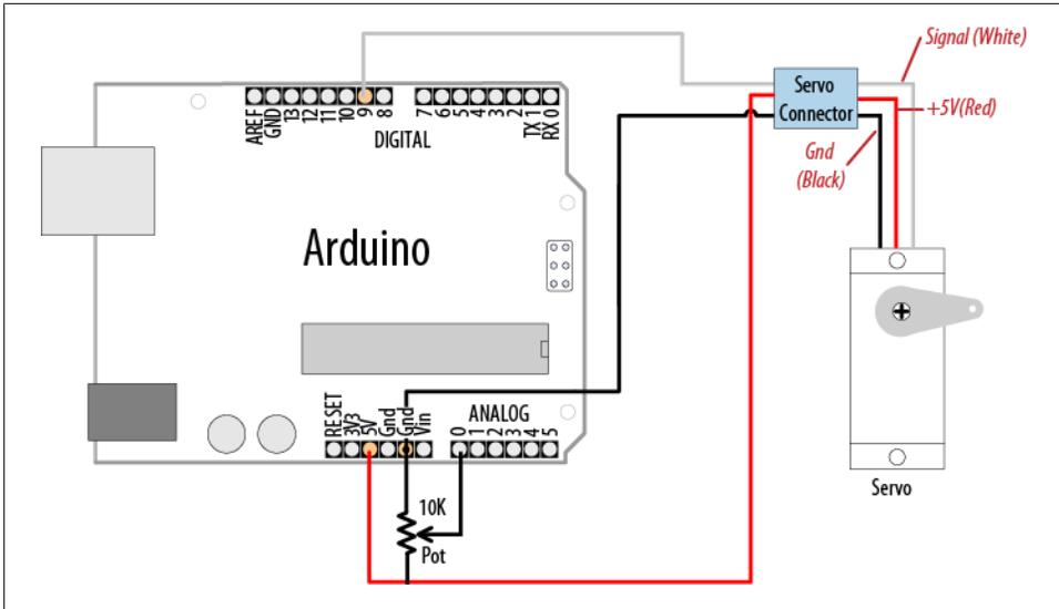
Figure 8-4. Controlling a servo with a potentiometer
