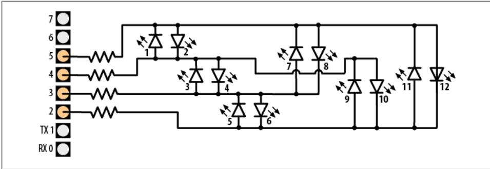
Figure 7-9. Charlieplexing using four pins to drive 12 LEDs
