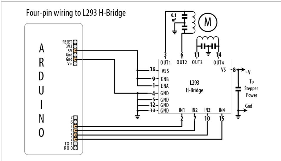
Figure 8-14. Four-wire bipolar stepper using L293 H-Bridge
