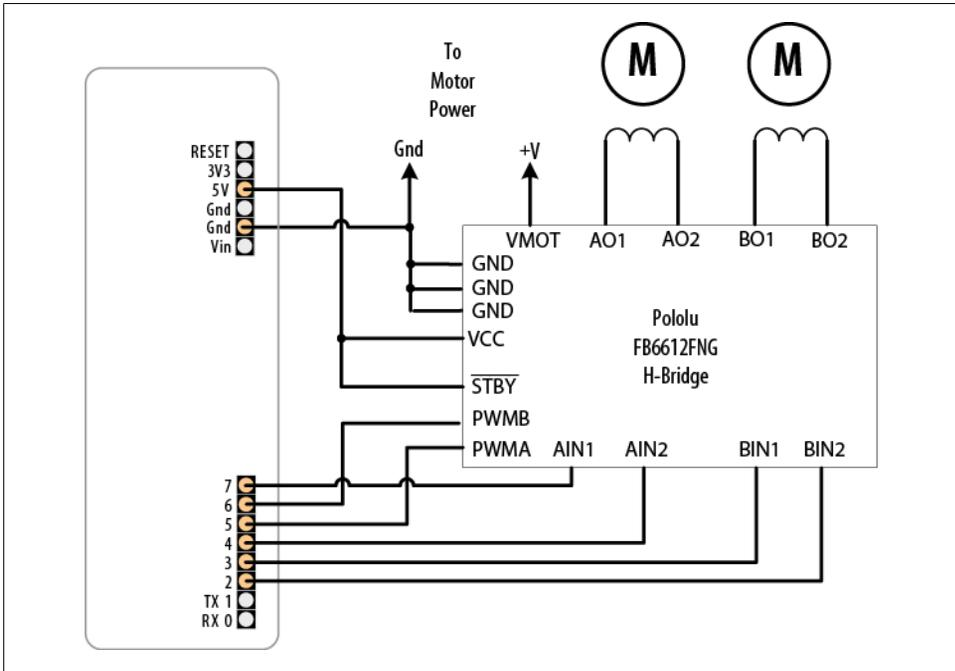
Figure 8-13. H-Bridge wiring for the Pololu breakout board
