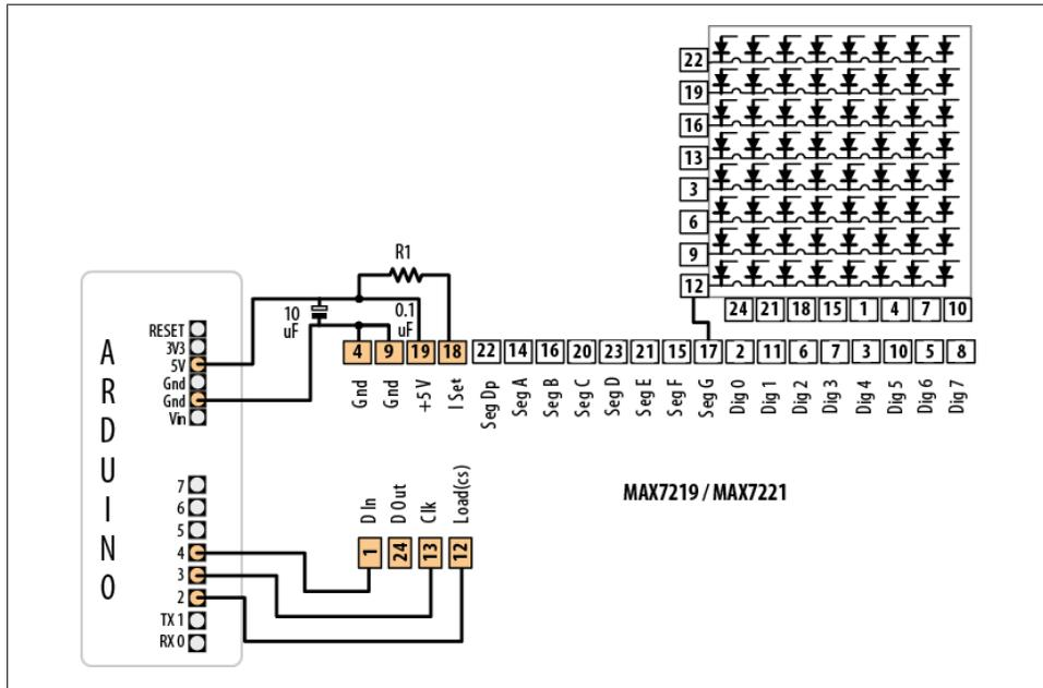
Figure 7-13. MAX72xx driving an 8x8 LED array
