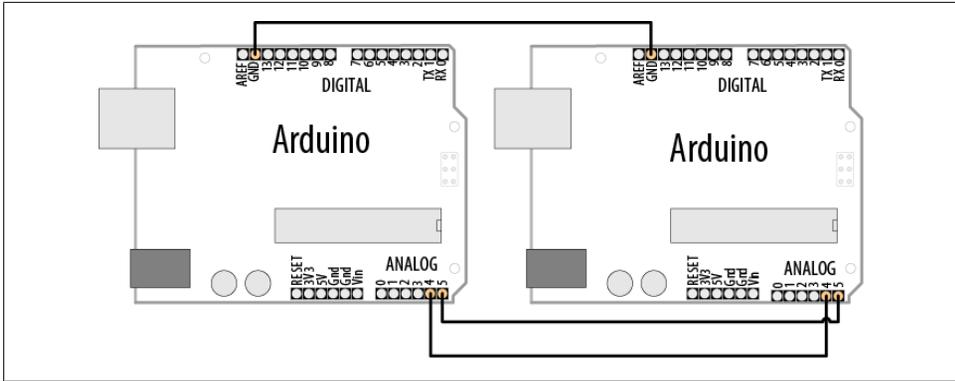
Figure 13-14. Arduino as I2C master and slave
