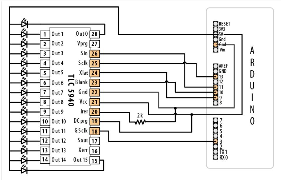
Figure 7-14. Sixteen LEDs driven using external PWM
