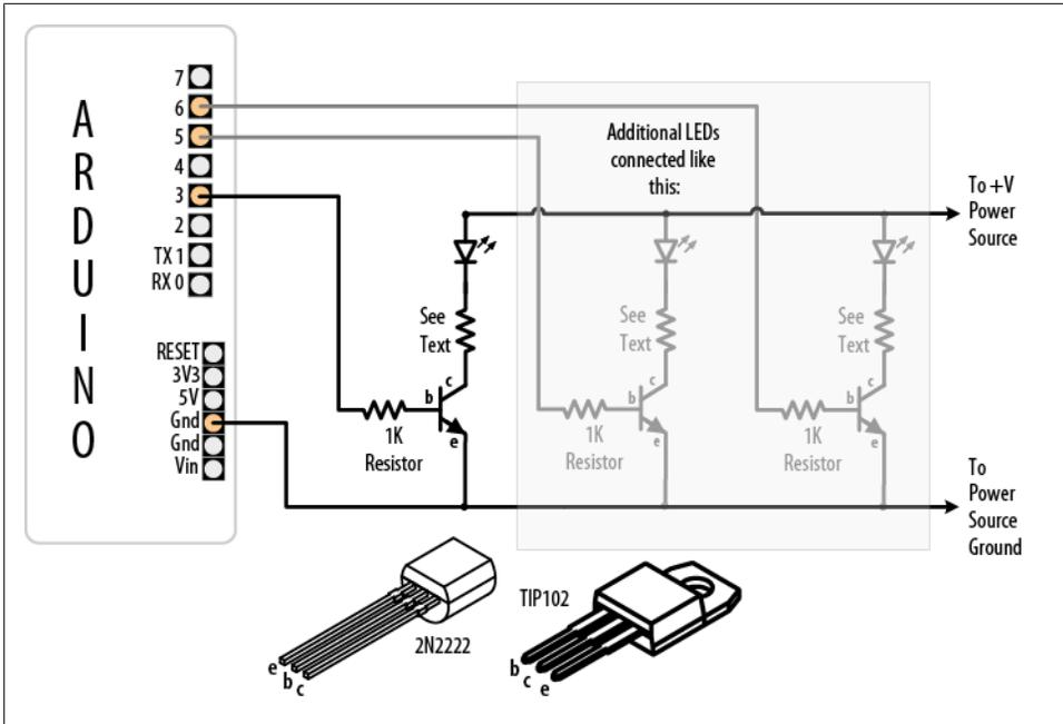
Figure 7-3. Using transistors to drive high-current LEDs
