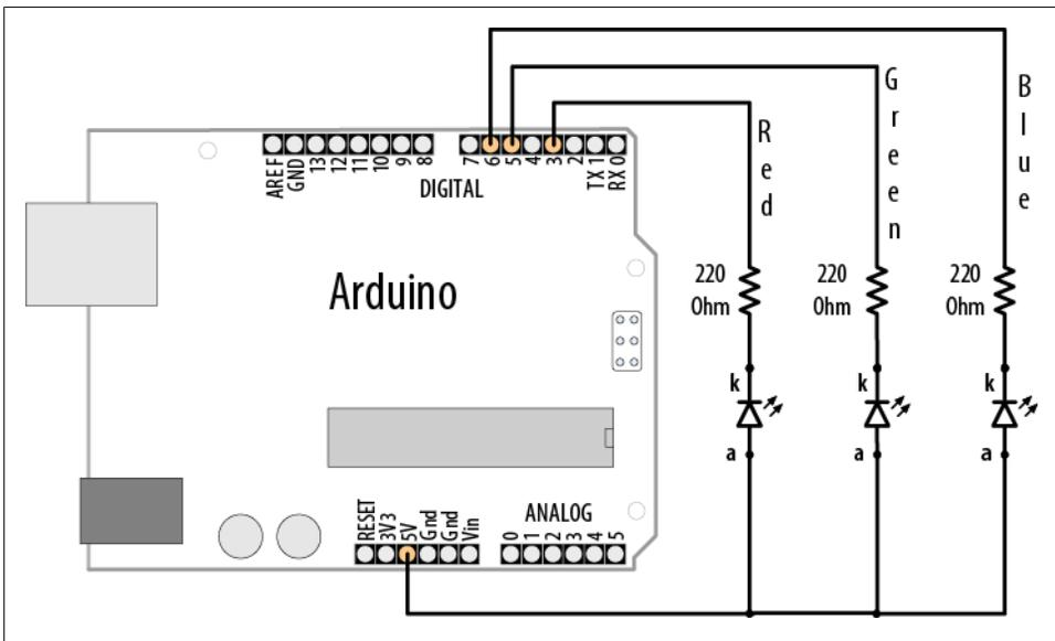
Figure 7-4. RGB connections (common anode)
