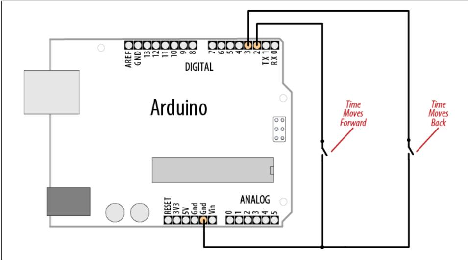
Figure 12-1. Two buttons used to adjust the time
