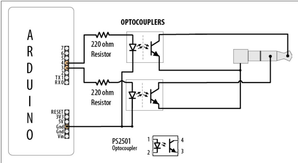
Figure 10-3. Using optocouplers with a TRS camera connector
