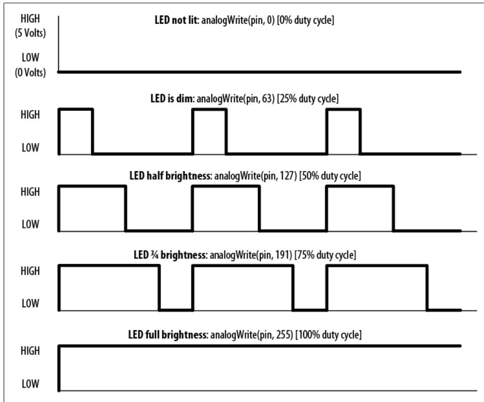
Figure 7-1. PWM output for various `analogWrite` values
