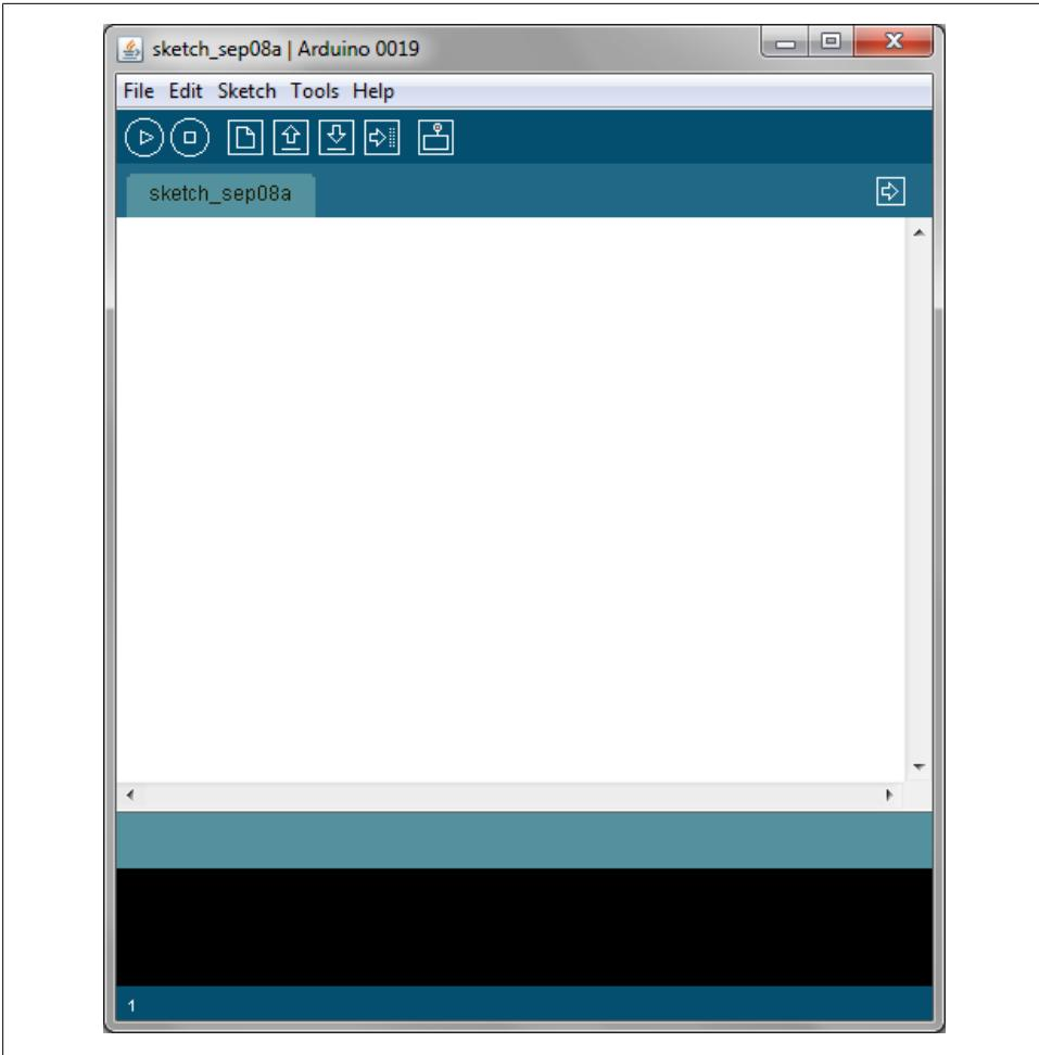
Figure 1-3. Arduino IDE main window (version 0019 in Windows 7)
