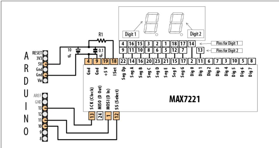
Figure 13-13. Connections for MAX7221 with Lite-On LTD-6440G
