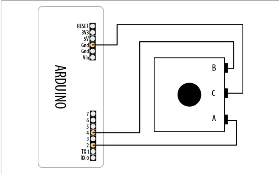
Figure 6-12. Serial RFID reader connected to Arduino
