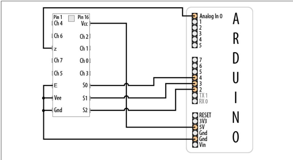
Figure 5-8. The 4051 multiplexer connected to Arduino
