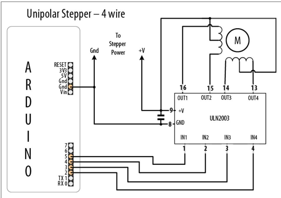
Figure 8-17. Unipolar stepper connected using ULN2003 driver
