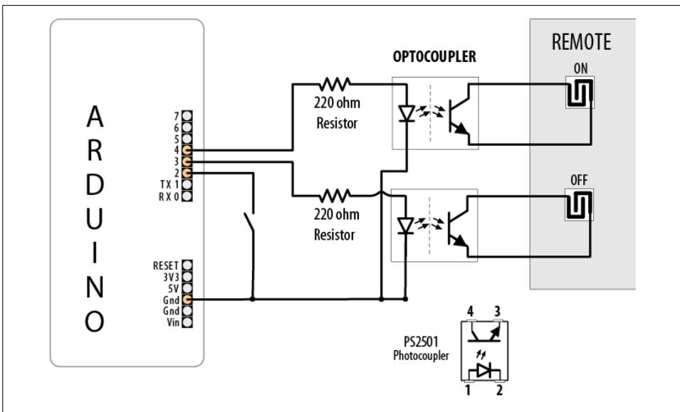
Figure 10-4. Optocouplers connected to remote control contacts
