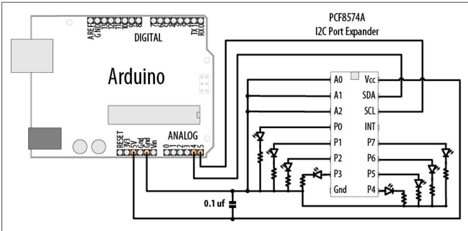
Figure 13-12. PCF8574A port expander driving eight LEDs
