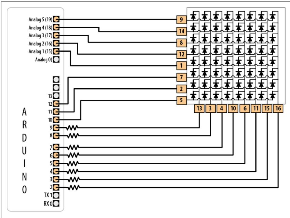
Figure 7-6. An LED matrix connected to 16 digital pins
