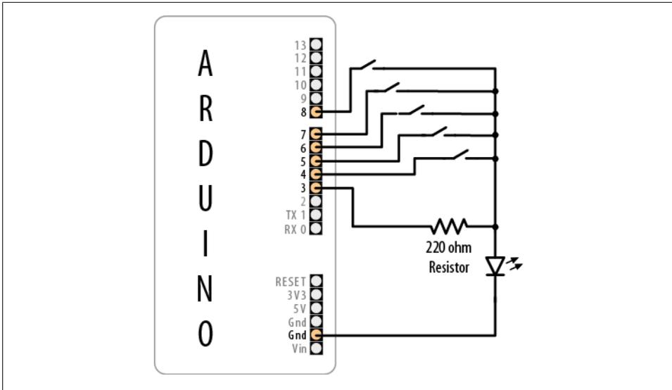
Figure 10-2. Buttons and LED for IR sender
